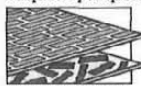
The pure chromium dioxide particles in the PRO II, unlike ferric oxide particles, are homogeneously shaped and uniaxially aligned to give this tape superior performance.
